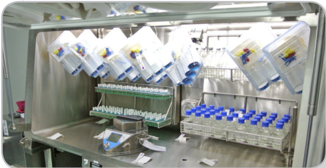
Customized interchangeable racking for sterility test batches
