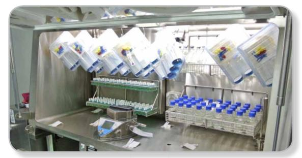
Customized interchangeable racking for sterility test batches
