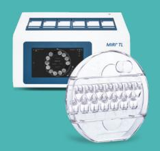
The lid is mounted inside the circumference of the dish covering the culture area completely – the user will only grab the dish during handling and not risk losing the dish by holding on to the lid only – as can be the case on all traditionally designed dishes. A large well is provided outside the culture are for pH measuring without affecting the cultured samples. The dish has a flat bottom so it is ideal for heat transfer from below.
